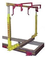
Car Bench unique specific jig portal is an extremely helpful tool for the repair on all the higher points of the vehicle. The specific jigs to be mounted on this system will ensure extreme holding of each jigging point.
