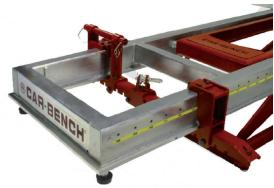
Car Bench Downward Pulling System with multi pulling features, the easiest way to carry out down pulling operations to lower the underbody to its original level, able to resist up to 3 Tons. For frames 180x100mm. This Car Bench downward pulling system is very sturdy and yet very easy to install on the frame before and after any pulling operation. Many different accessories can be used on this repair system.
