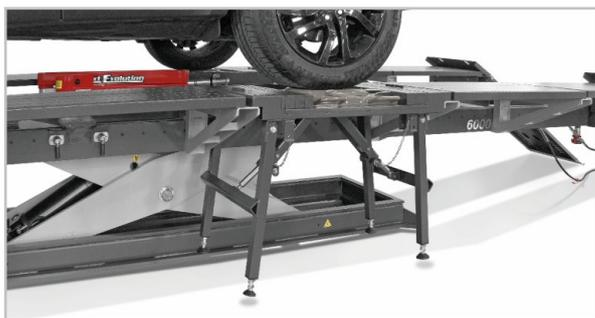
DES SUPPORTS D'ALIGNEMENT UNIQUES PERMETTENT UN NIVELLEMENT PARFAIT DU VÉHICULE
