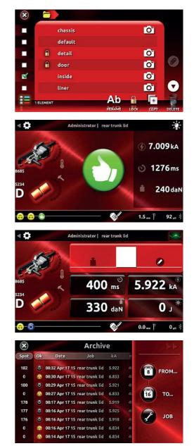
**New touch screen welding control unit** with intuitive graphic diagrams, allowing a very simple use of the machine by the user.
